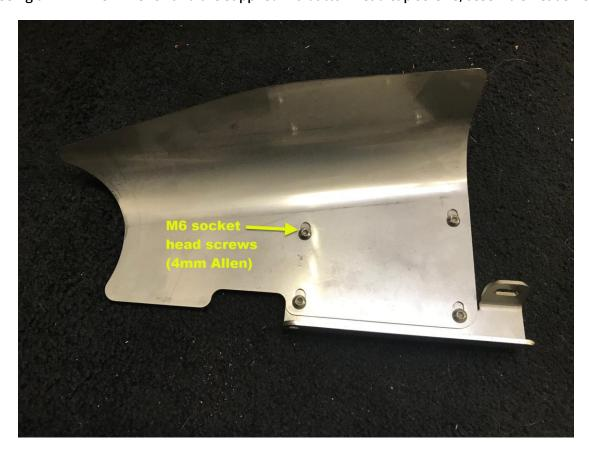
Step14 - Install the heat shield by attaching to the stock inlet tube mounting bracket (Step 6), and the head sensor (Step 12). Shield location can be adjusted by loosening the M6 button head cap screws. Make sure wiring along the firewall does not contact the edge of shield.
