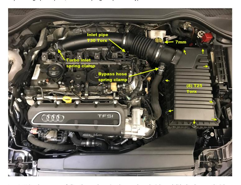
Step 4 – Using the same set of pliers, loosen the spring clamp at the turbo inlet and slide the clamp up the inlet pipe and off the coupler (see image in Step 3).
