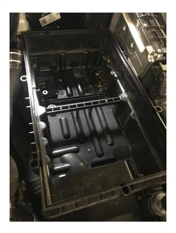
Step 10 – Using the supplied hobby saw, remove the OE air filter center support.
