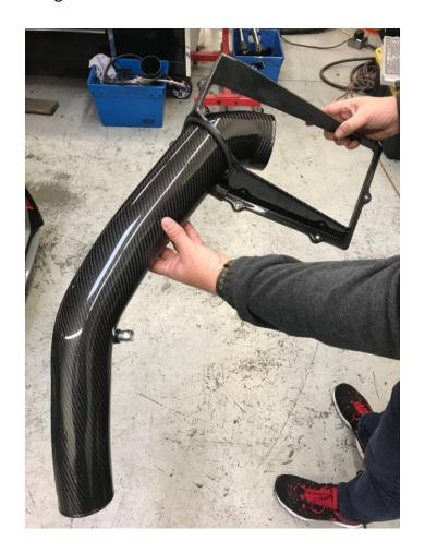
Step 17 – Rotate intake tube within airbox frame and install the air filter. Using an 8mm socket, tighten hose clamp. NOTE: Do not over-tighten, as this may damage the carbon tube. It does not have to be very tight, just snug.
