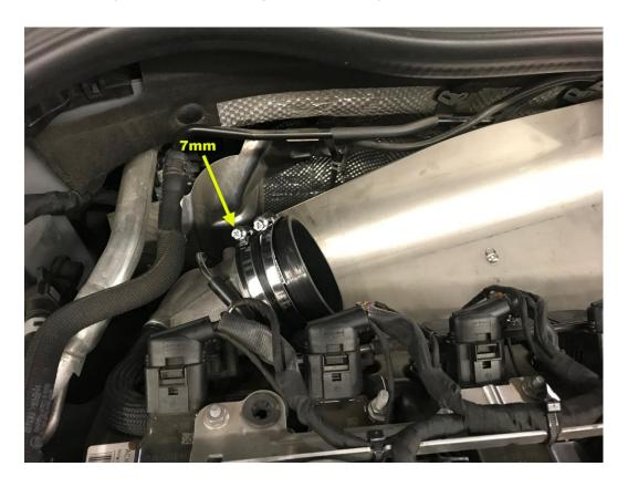
Step 16 – Insert intake tube through the hole in the carbon fiber airbox frame.
