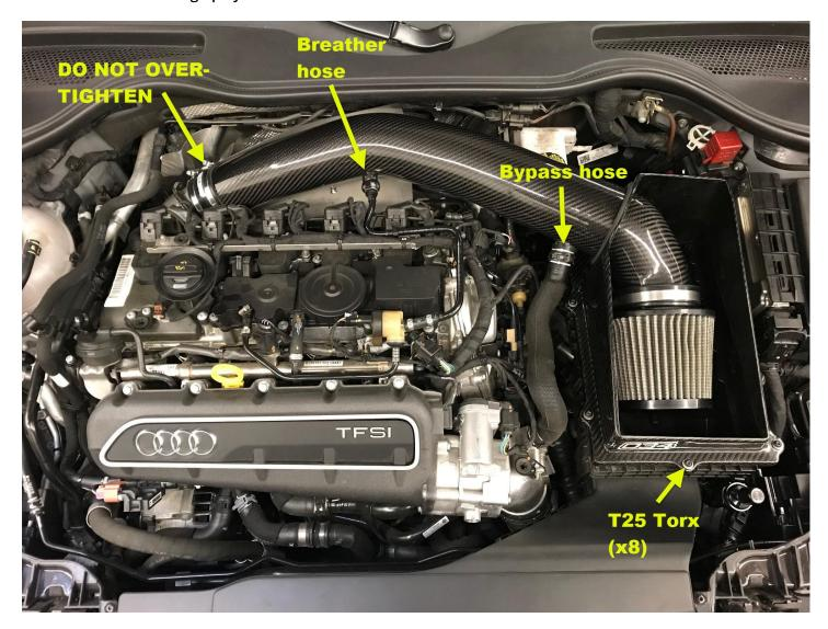
Step 20 – Connect breather hose (removed in step 11) to intake tube fitting. It will snap on when fully seated (see image in Step 19).
